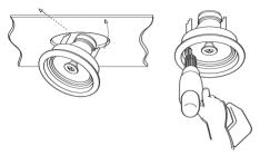
5. Adjust the direction of the speaker by swiveling it to the left or right as needed. If desired, you may also adjust the tilt of the speaker and gently adjust the horn to the desired angle. Do not attempt to turn the tweeter stem while adjusting the swivel tweeter.
